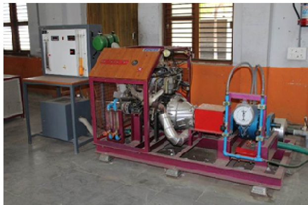
Multi cylinder 4 stroke petrol engine test rig with hydraulic dynamometer (MPFI) with Mohr's test
