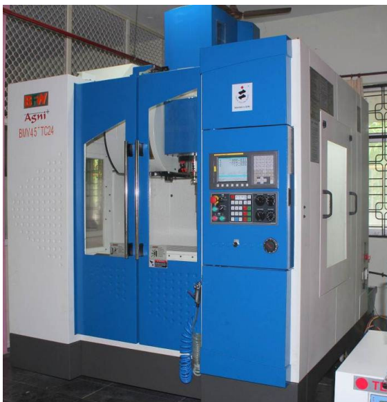
Vertical Machining Centre (Make: Bharat Fritz Werner)
